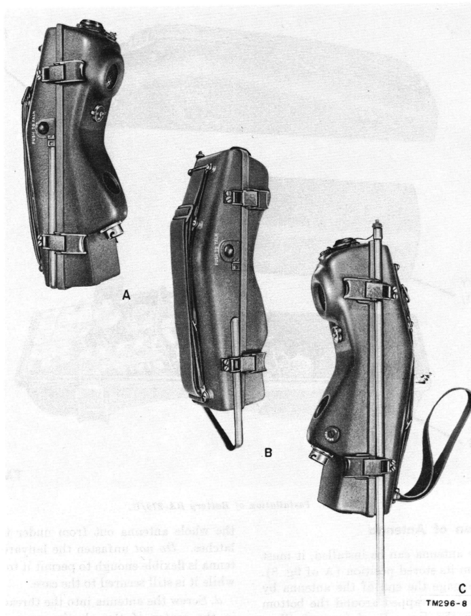
Figure 8. Installation of antenna.
